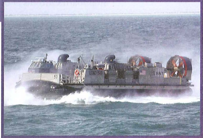
The LCAC travels across the water on a cushion of air. Courtesy of the US Navy
