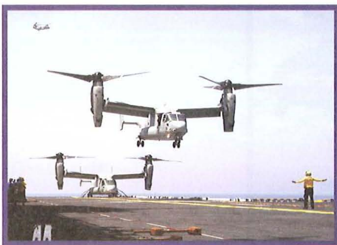
The V-22A Osprey is a helicopter that turns into a turboprop plane.
