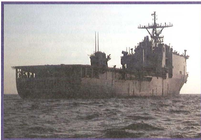
Dock landing ships such as USS Carter Hall carry and launch amphibious craft and vehicles as well as crew and troops.
